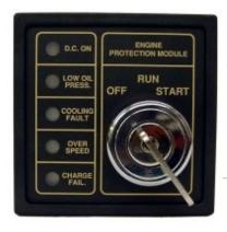
Combining the convenience of manual operation with engine protection against Low Oil Pressure (LOP), Coolant Fault(HET) and (optionally) Overspeed and an Auxillary Input, these Keystart Modules are easily mounted into almost any control panel or switchbox. Set in a compact 72mmsq DIN sized module they can be used with a wide range of engine driven equipment. Five 'High Intensity' LED's indicate system status.
