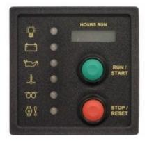
This micro-processor based controller directly replaces the earlier PSM72. It allows manual start - stop in bad weather conditions that a conventional keyswitch could not provide. Timed Pre-Heat with LED indication together with engine protection for Low Oil Pressure, Cooling Fault and Over-crank. Customised versions and customer specific software is available to order. Note: the PSM720 shares the same connections with the ASM720 series
