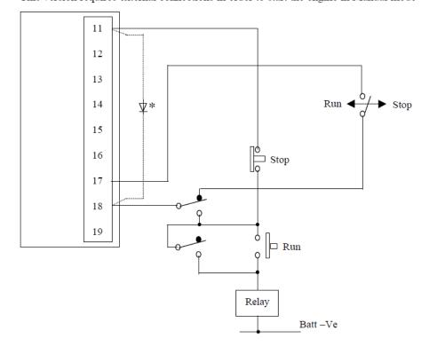
Note: Fit diode (\*) as shown if 'Stop / Start' circuit not used and connect 'Run / Stop' volt-free contacts from term.17 to 18 as standard.
