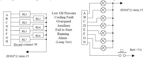
4/ RSM72--T-- 'Active-Low' driver output (on term.7) at the end of the 'T0' hold-off timer period
