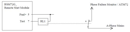
The (open collector transistor) Test output (term7 above) switches to battery -Ve (active-low) when the engine has achieved crank-cut speed with no fault shutdown present and 'Test' mode selected.
