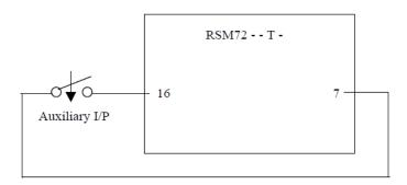
Connected as shown above, the 'Aux.' channel is subject to the 'T0' timer, and provided with 'First-up Interlock'. This 'T0' output is capable of sinking 300mA / 30VDC and could be used to drive an external relay (connected to term.15).
